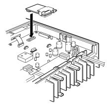
⑥ Replace the bottom cover and screws, then the DC power cable.
